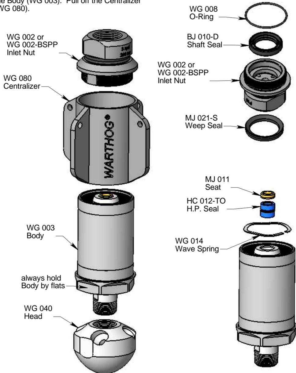
3. Remove the O-Ring (WG 008) and Weep Seal (MJ 021-S) from the Inlet Nut.
