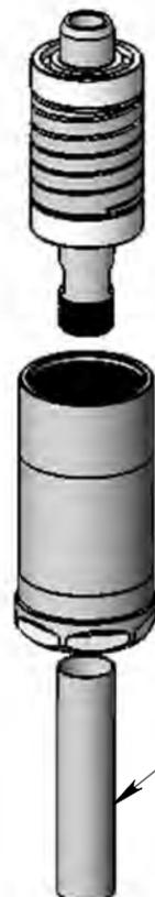
5. Place the Wave Spring (RJ 014) on top of the Bearing. Add more viscous fluid until the Wave Spring is covered.
